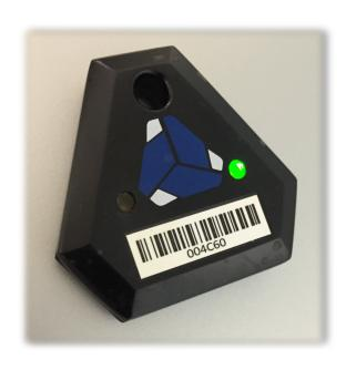
Visybl is making that solution possible through the use of Bluetooth Low Energy (BLE), technology that is supported in most Apple and Android smartphones. Our BLE-based AssetBeacon turns your physical assets into tiny sensors, continuously transmitting information about their presence, temperature, movement, for years on a single battery.
